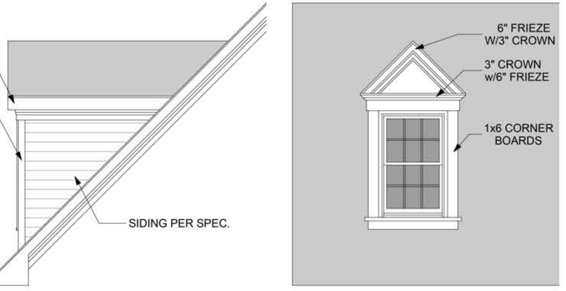
-typical dormer detail- -scale: 3/8" ===== 1'-0"-
